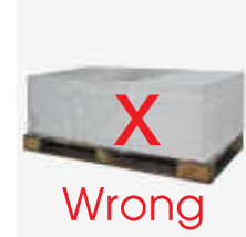
A part of the pile is not covered by plastic film
