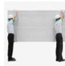
When moving, DURAflex should always be lifted edge-up, with the board width oriented vertically.
